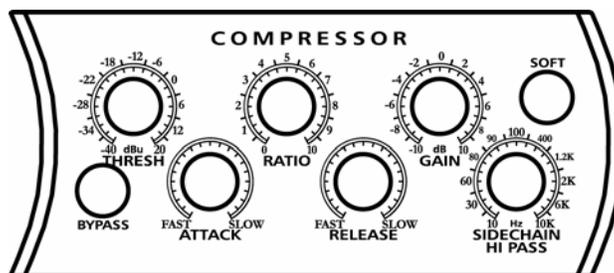
**THRESHOLD:** Sets the level at which compression begins. When the signal is above the Threshold setting, it becomes ‘eligible’ for compression.
